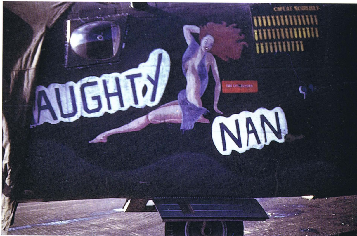
Naughty Nan was another 446th Bomb Group Liberator, a B-24H with the 705th Squadron. She made it through quite her share of combat, as the bomb symbols attest, but was written off after a local hop and a forced landing at Bungalow when the right landing gear leg wouldn't come down. Albert R. Krassman
