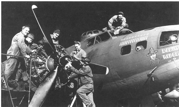
ABOVE Unsung groundcrew. The ground and maintenance crew of B-17F DELTA REBEL NO. 2 service the number three engine between raids. Sgt Maurice Gole, crew chief, is examining the propeller hub. This photo was taken in the western end of the hangar used by the 323rd BS/91st BG at Basingstoke during February 1943
