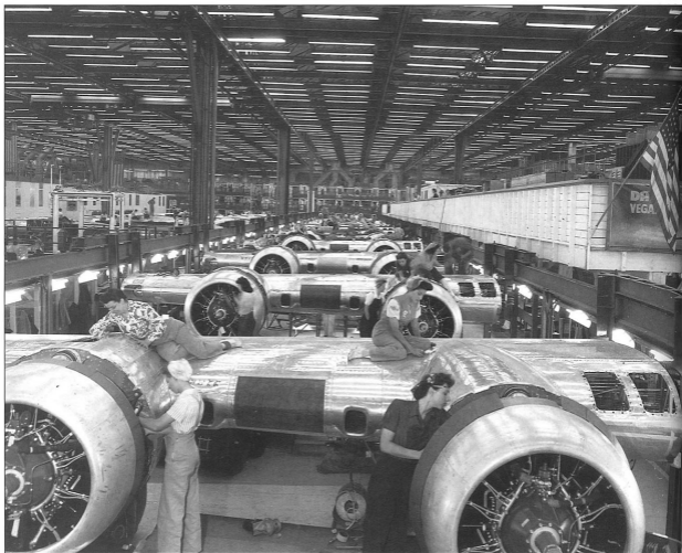
Seemingly never-ending B-17G wing sections head down the Vega production line
