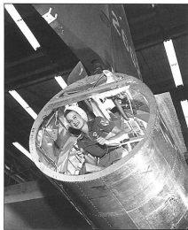
A Vega worker is seen installing wiring prior to the attachment of the tail gun position, which was built as a separate component
