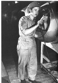
ABOVE A Boeing worker rivets on a long line of tail gun positions. Note the suitably stylised company uniform
