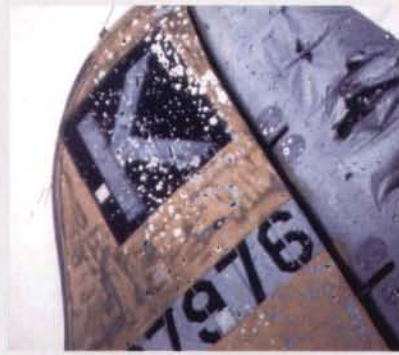
The flak damaged tail section of 'A Bit 'O Lace' affords a close-up view of the 'Square K' emblem and aircraft identification numbers with small unfilled stencil lines. Note the unpainted metal replacement rudder, soon to be replaced once again.
