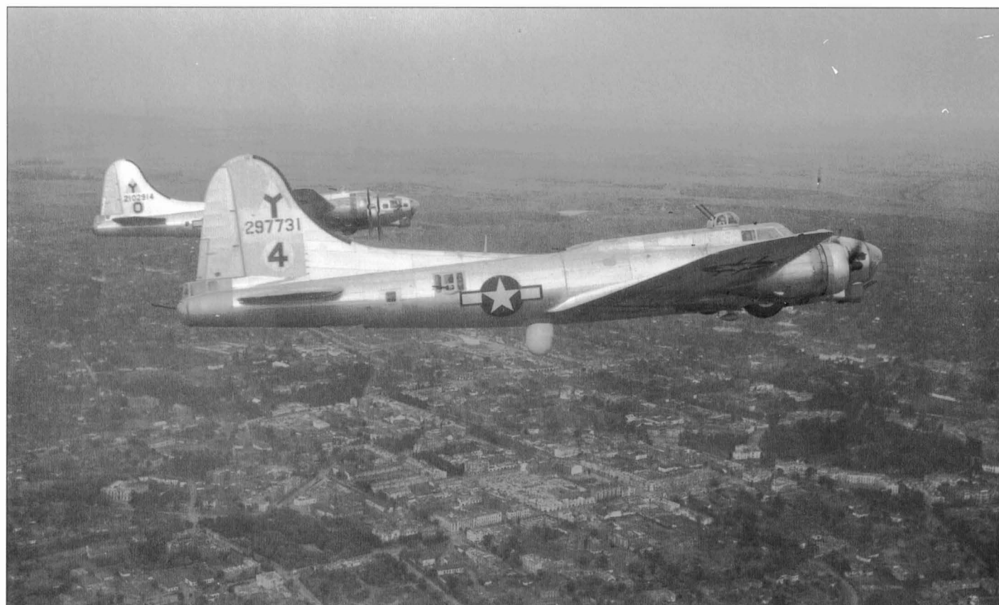
Above and below are unnamed B-17s of the 97th Bomb Grp., Fifteenth Air Force. Note the unique, late model, radar dome in place of the belly turret on #297731.
