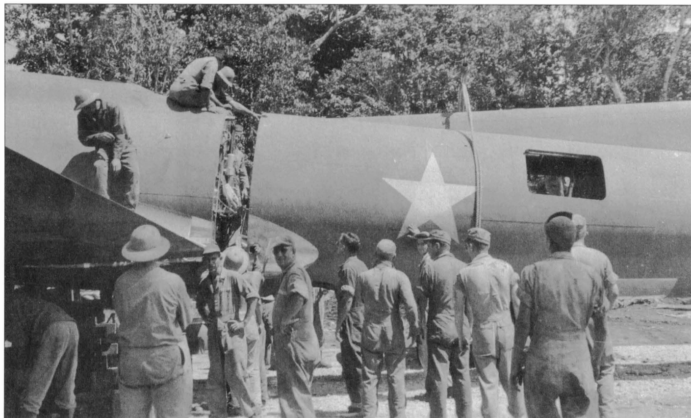
These unnamed B-17s of the 11th Bomb Grp. (probably 26th Sq.) are shown on Guadalcanal in 1943, operating with the Thirteenth Air force. It seems likely that the crude wedding of the tail section (below) with the nose was part of a major job of cannibalization.
