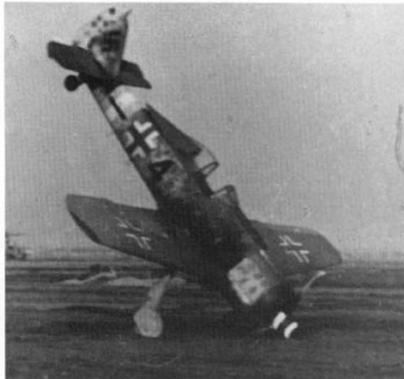
"Black 4," a Fw 190A-8 of 8./JG 300 after a misjudged landing. It had a blown canopy, no additional armor, and recently introduced blue-white-blue rear fuselage bands. It was flown by Lt Viki Helmann. Note the Mistel in the background.
