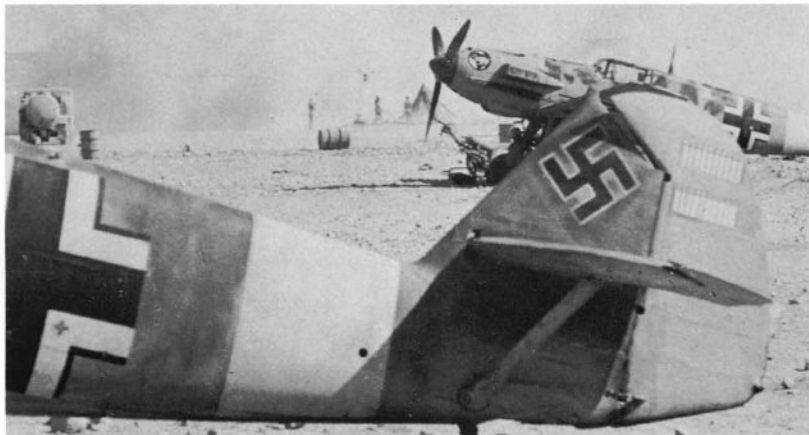
Above: Two Bf 109Es of I/JG 27 photographed in the Western Desert during 1941. The machine in the foreground appears to have been lightly oversprayed and shows twenty victory bars on its rudder. Behind it was a Bf 109E-4/trop with freshly applied field camouflage in sand yellow 79, and brownish-green 80 mottling over pale blue-grey 65, a scheme later adopted by the entire Gruppe . Below: Bf 109F-4/trops of JG 27 in the later colors of tan 79 upper surfaces over 78 sky blue in conjunction with the usual white theatre markings.
