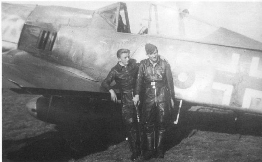
Fw 190A-8/R8, "Red 8," Pimpf , of Mattäus Erhard, the Rottenflieger (wing man) of Bretschneider of 5./JG 300. Left: Erhard, right Ernst Schröder. Note that the MG 131 openings are covered.
