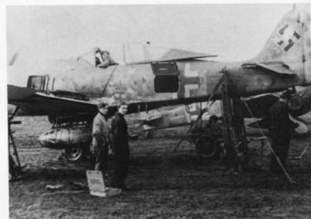
Above: A busy scene with "Yellow 1" lifted at its jacking points. This and the aircraft behind it are believed to have had red rear fuselage bands.
