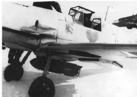
This Bf 109E, "White 1," armed with a 250kg bomb, is believed to have been the aircraft of the well-known Waldemar (Hein) Wübke. At the time it had five victories on the rudder.
