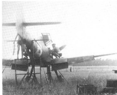
Bf 109E, "Yellow 10," in Russia. Dark camouflaged aircraft under weapon aligning exercises.
