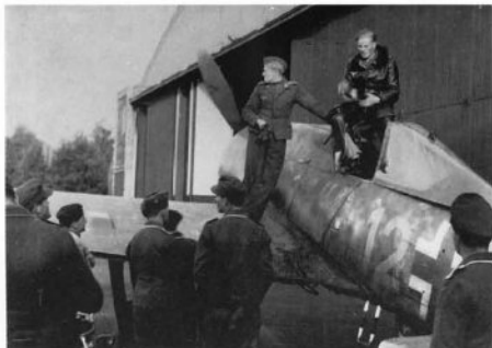
Two views of "Yellow 12" a Fw 190A-8/R8 of Werner Bohnenkamp of 6./JG 300. This anti-bomber version was fitted with extra armor and two MK 108 wing cannons for close-in fighting.
