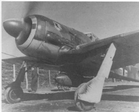
Fw 190 Jabo of I./JG 54 with 250 kg bomb. During long periods, there were not enough enemy aircraft in the air, so the fighters flew ground attack sorties.
