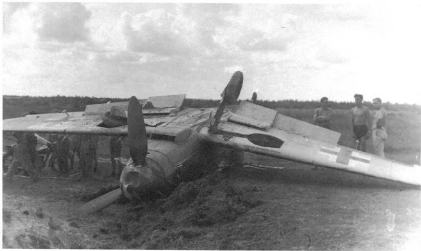
The pictures on this and the opposite page are of Bf 109G-1, "Black 1", of 9. Staffel which crashed down near the airfield. The pilot was the famous Walter Nowotny who had shot down three aircraft on this mission. He "buzzed" the airfield three times for three victories, but in the last turn he ran out of fuel, causing this accident. Nowotny wasn't hurt at this time. Note that the aircraft was repainted in a dark-green color similar to 71. Airfield was Rjelbitzy during November 1942.
