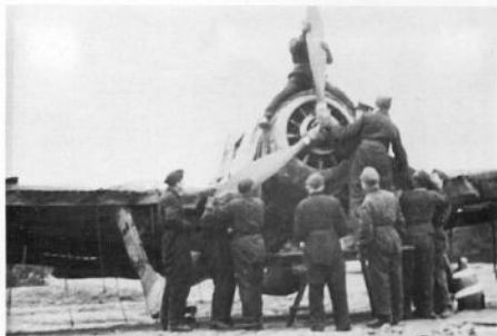
Propeller exchange on a Fw 190 of JG 300.
