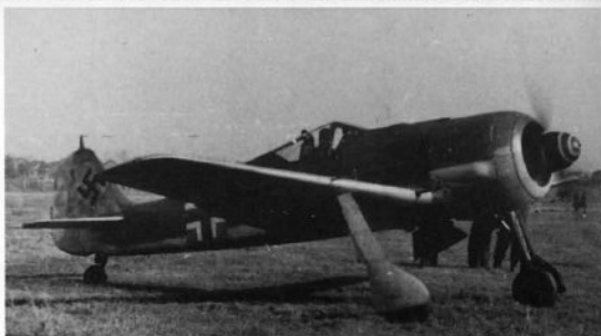
Note: Outerwing guns of Fw 190A-6 removed.
