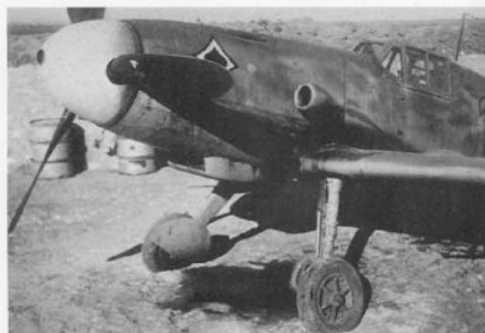
Bf 109G-2, "Yellow 13," of 3./JG 53, photographed somewhere in North Africa. The fighter was not fitted with the usual sand filter.
