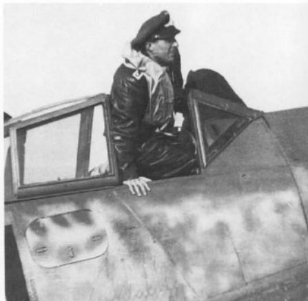
Above: This Fw 190A-8/R8, "Black 8," was flown by Ofw Richter who is photographed here during a lull between bombing raids. Additional armor was fitted to the sides of an otherwise standard cockpit. This "Black 4" should not be confused with that flown by Viki Heimann.
