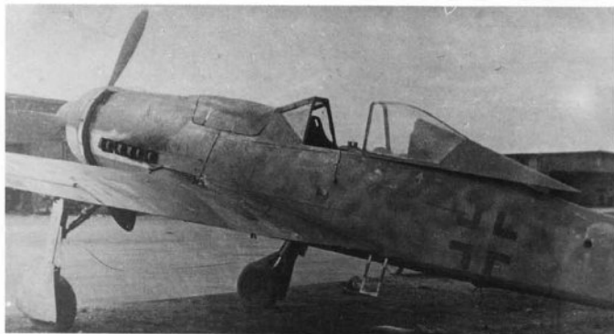
Left and below: This Fw 190D-9 was used by the staff of JG 301 and had a yellow lower cowling, plus an oversprayed swastika. Note the ETC bomb racks used for ground-attack operations in the closing weeks of the war.
